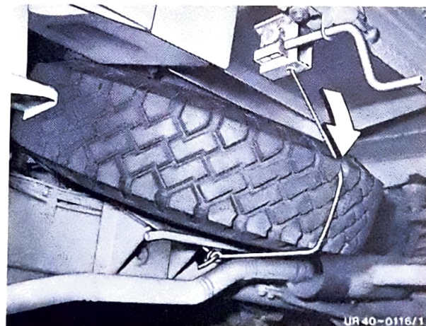
Release spare wheel and lower with crank
