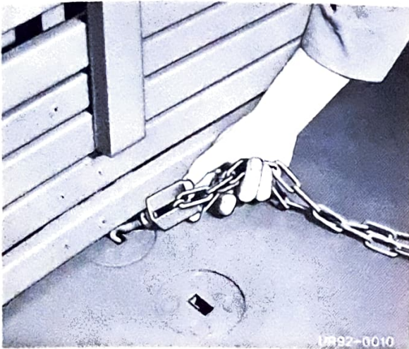
Insert tensioning chain in platform hole
