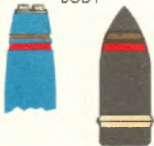
FIG.7 CAST IRON OR SEMI-STEEL BODY
