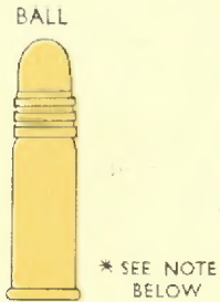
FIG.1 CARTRIDGE, RIMFIRE, .22 INCH
