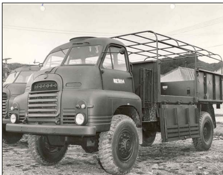
The Bedford RL was the New Zealand military's main medium truck from 1958 to 1989. For more info see the back page.
